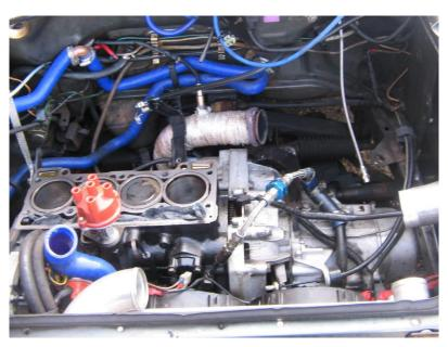
Once removed use your solid steel rule to check to make sure the head is flat and not warped so from 1 corner to another and across make sure there are no gaps or signs of warping on the head. Do the same on the block. If your head is warped either replace it with another or get it skimmed professional by a local engineering firm.
