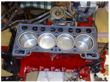
If the head is all clean and checked for flatness place it carefully and slowly on top of the new head gasket making sure the alignment hole is aligning with the H/g and the hole will slot into the head slightly and then leave the head in place.
