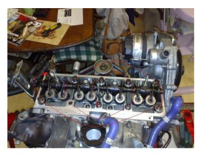
OE Head bolts & OE Head gasket **60 NM** Meillor Blue Seal Head gasket and 12.9 High Tensile Head bolts – **80NM** (can be tightened any where from 65-90nm).
