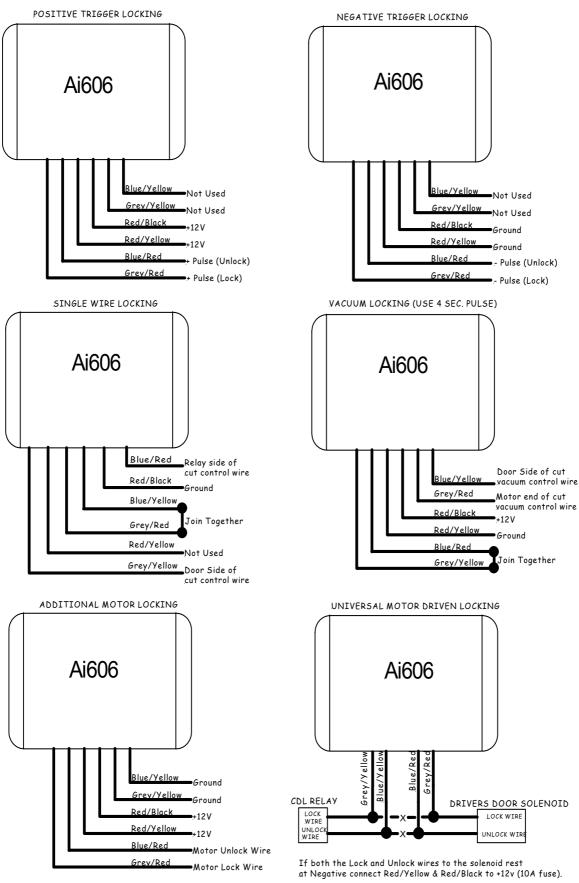
If both the Lock and Unlock wires to the solenoid rest at Positive connect the Red/Yellow & Red/Black to the vehicle Earth.
